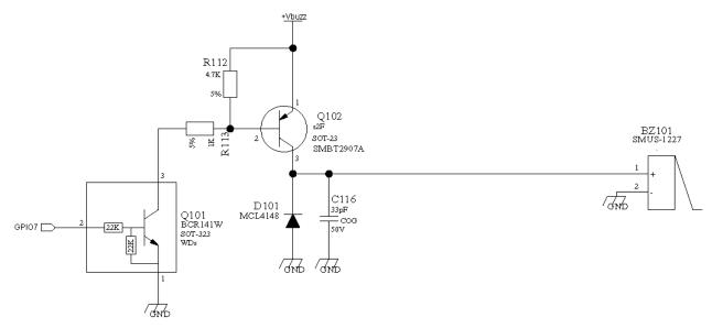
NOTE: To correctly drive a buzzer a driver must be provided, its characteristics depend on the Buzzer and for them refer to your buzzer vendor.
