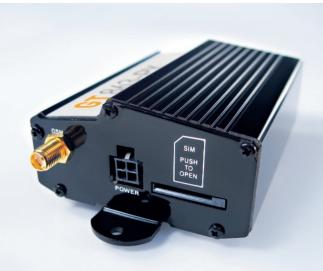
The Telit GT863-PY terminal is a complete encased modem solution for wireless m2m applications.
