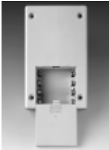
Battery compartment of case sizes 155, 190 for 4 mignon cells 1.5 V (AA) or 2 flat batteries 9 V (PP3). (Clips for AA cells fitted)
