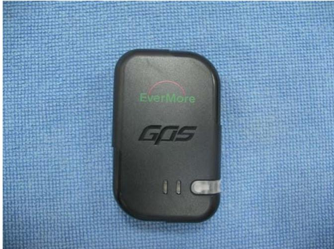
**The BT-R800 is a GPS receiver with Wireless interface and built-in Patch antenna for high sensitivity to tracking signal.**
