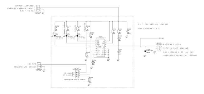
NOTE: In this particular application the battery charger input current must be limited to less than 1A. This can be done by using a current limited wall adapter as the power source. For your convenience in the EVK there's also a current unlimited input, where the input source is not limited in current and the drawn current is limited to about 0,5A by a MOSFET in the EVK.
