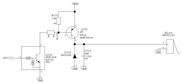
A sample interface scheme is included below to give you an idea of how to interface a Buzzer to the GPIO7:
