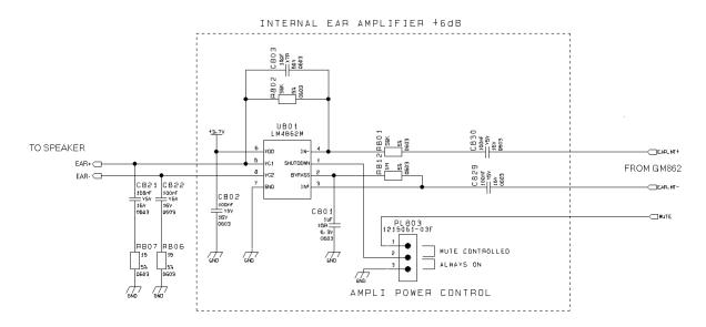
Some amplifier require a low impedance load at high frequency in order to avoid auto oscillation, this can be made with a capacitor (100nF) in series with a resistor (15 $\Omega$ ).
