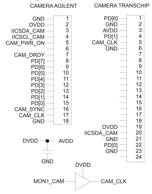
The numbers on the left side of the Camera's connectors refers to Module Connector's pin number. DVDD is an external power supply of 2.8V, controlled or gated by pin CAM\_PWR\_ON.
