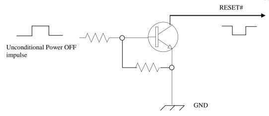
NOTE: don't use any pull up resistor on the RESET# line nor any totem pole digital output. Using pull up resistor may bring to latch up problems on the GM862-QUAD power regulator and improper functioning of the module. The line RESET# must be connected only in open collector configuration.
